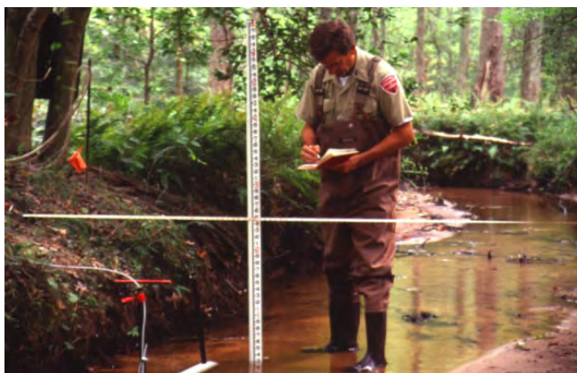
Figure 11: Measuring bankfull stage
